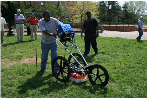
Troy General demonstrates ground-penetrating radar.
